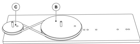
Turn  ${\bf C}$  pulley in one direction of rotation and note on drawing the direction of rotation of  ${\bf C}$  and  ${\bf B}$  pulleys.
