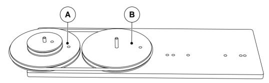
Turn the A pulley in one direction of rotation and note with arrows on drawing the pulleys A and B direction of rotation.
