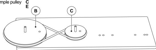
Turn  ${\bf B}$  pulley in one direction of rotation and note with arrows on drawing the direction of rotation of  ${\bf B}$  and  ${\bf C}$  pulleys.
