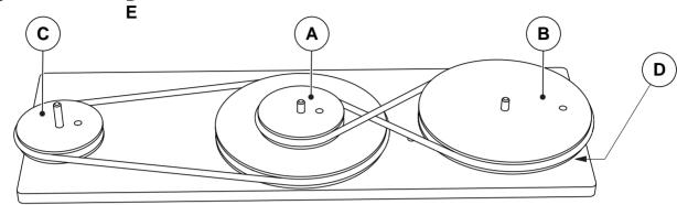
Turn **C** pulley in one direction of rotation and note with arrows on drawing the direction of rotation of C, A, B pulleys.
