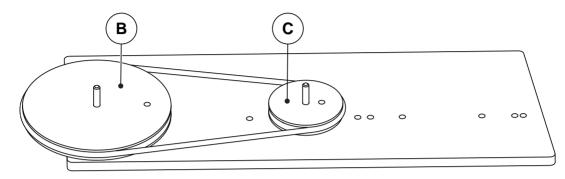
Turn B pulley in one direction of rotation and note with arrows on drawing the direction of rotation of B and C pulleys.
